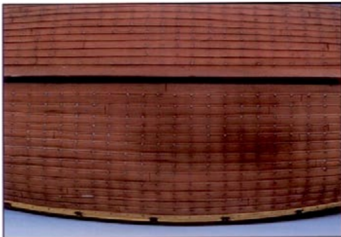
General view of the hull, with the subtle shading of the nails and the reddish colour of the planks after washing and dry-brush treatment.
