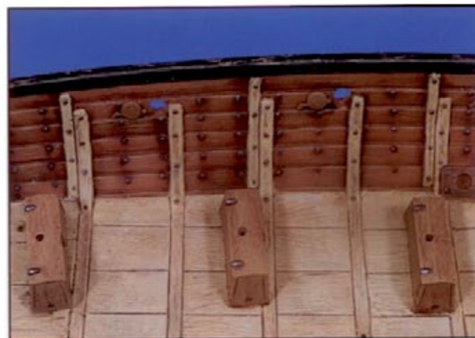
To paint the rail, we will follow the same steps used in painting the hull, as it is the same kind of reddish wood. It will be necessary to retouch the contact area between the rail and the deck. The scrapings on the upper black timber will add a touch of realism.
