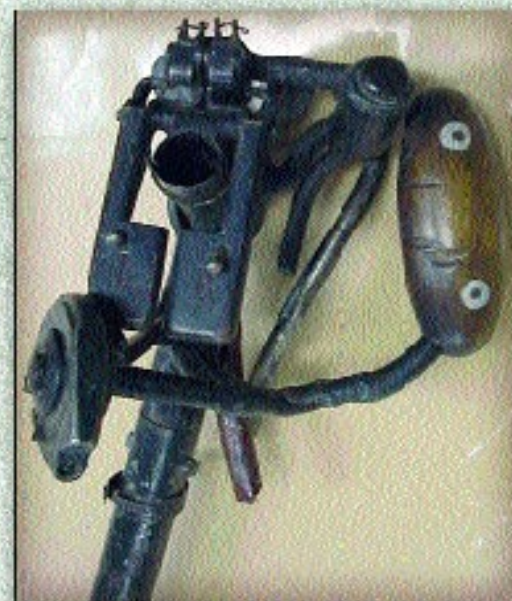
Von Richthofen's Fokker Dr.1 control column. Note the two triggers marked 'L' and 'R', for firing the LMG 08/15 machine guns.
