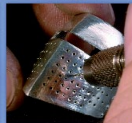
Drilling ventilation holes
