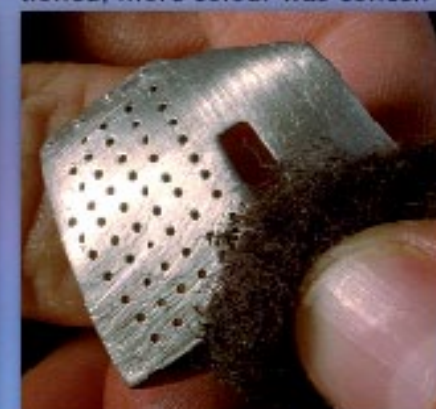
Polishing the part using steel wool
