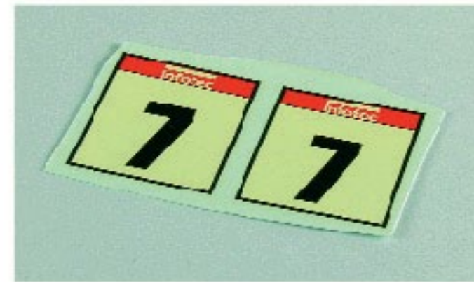
A typical example of decal damage: colour changes and cracking.
