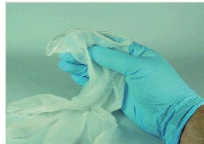
Vinyl or nitrile gloves are indispensable for avoiding paint stains or preventing the transference of contaminants to painted surfaces.
