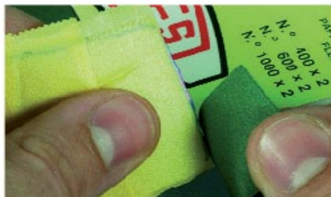
The part is masked with tape to protect it from possible mistakes and the remaining material sandpapered.
