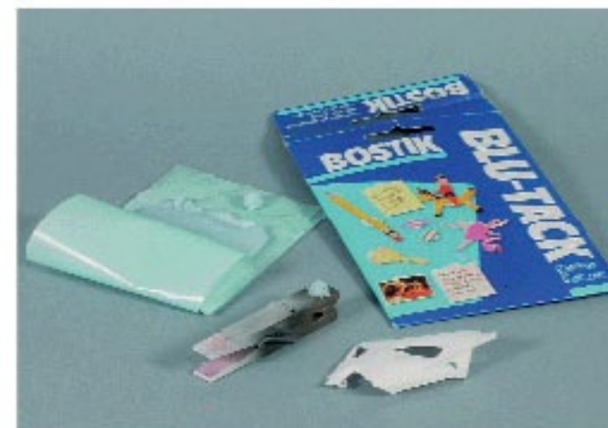
'Blu-Tack' is a very practical item for holding parts throughout the painting process, or as a mask, as it will not 'lift' the paint and leaves no residue when removed.
