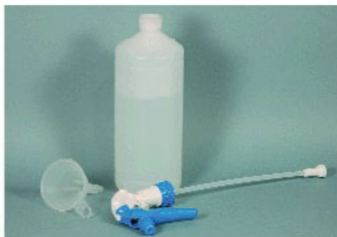
A spray bottle filled with water is useful both for cleaning and for 'wetting down' an area so that specks of dust are prevented from contaminating a part that is to be painted.
