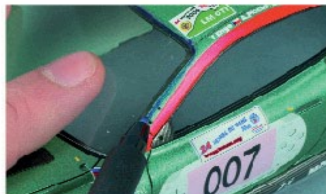
The part is placed in position and the surplus marked with a felt pen.
