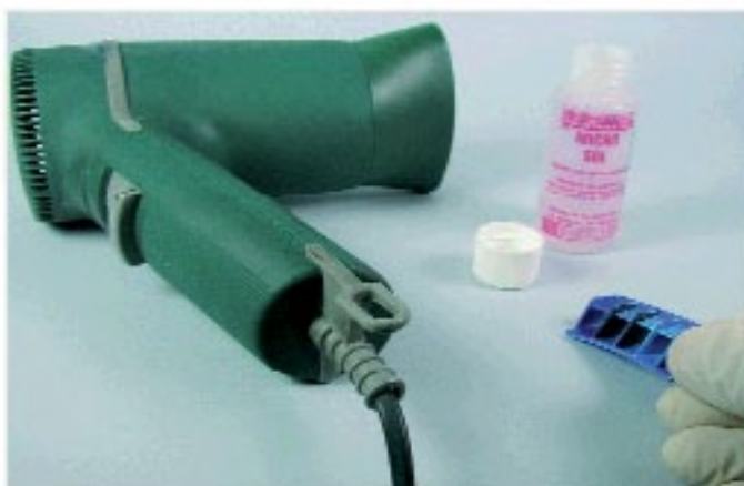
Drier used when applying decals. It can also be used to accelerate the drying time of paint.
